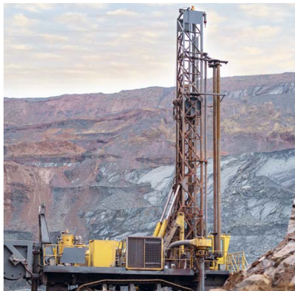
Large drill rig prepares boreholes for explosives in a quarry.
