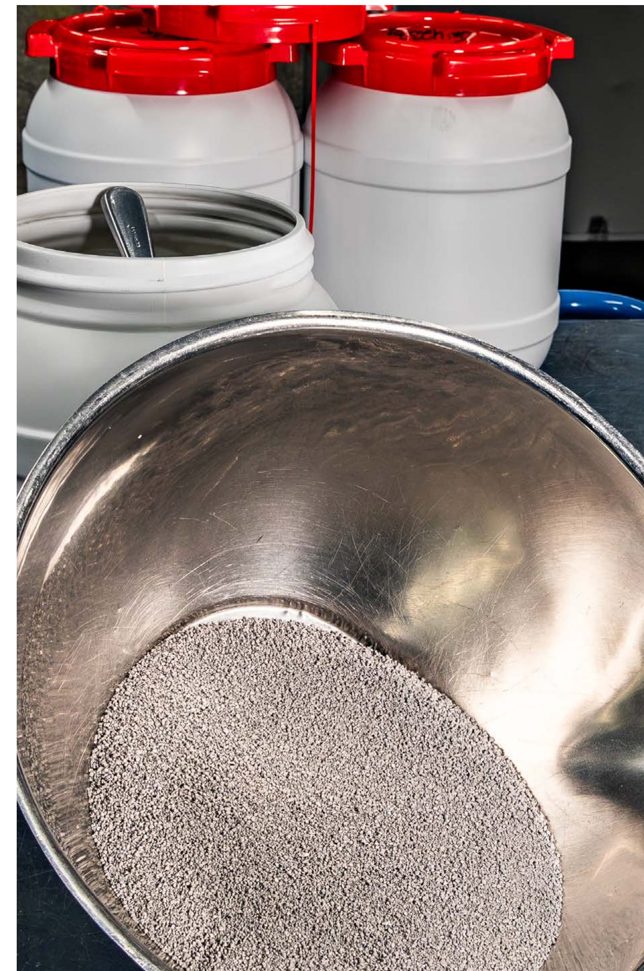
Figure 2. Platinum sponge, used in the manufacture of industrial applications. For pharmaceutical products, rigorous quality control and analytical testing are applied to ensure the highest standards of purity, quality.
